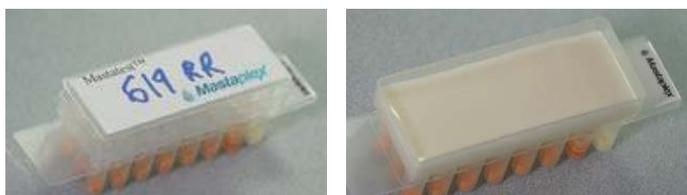
Mastatest cartridge with lid      Cartridge loaded with milk
