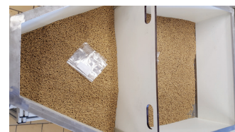
The cooler (Top view - cold air blown from bottom)
