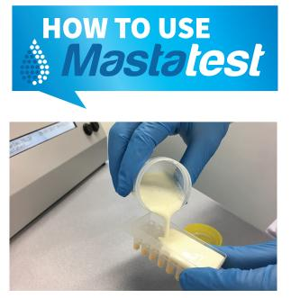
Fill the Mastatest cartridge with the milk sample (half full or holes are just covered)
