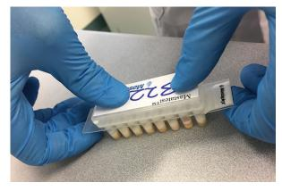
Tap the closed Mastatest twice to ensure the liquid is at the bottom of the wells
