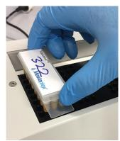
The Mastaplex label should cover the gap. Enter the cow ID and quarter infected, then start the test
