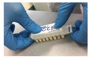
Tap the closed Mastatest twice to ensure the liquid is at the bottom of the wells. Pour excess milk sample back into the sample container
