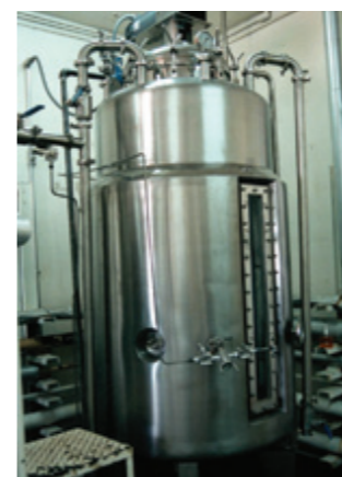
Picture 1: submerged fermentation is a liquid process taking place in a fermentor
